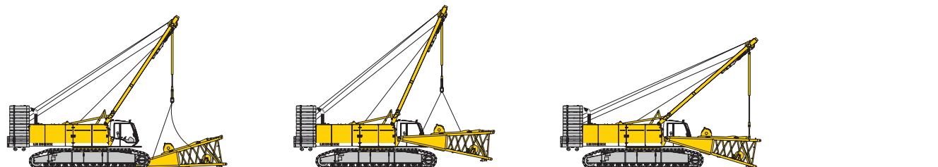
Unloading and assembly of boom foot
