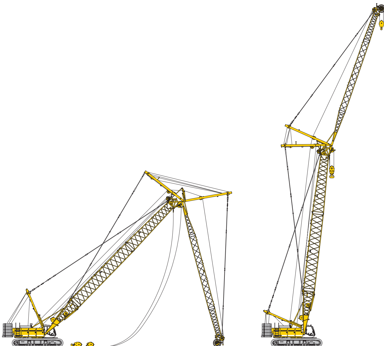
Erecting of main boom and luffing jib
